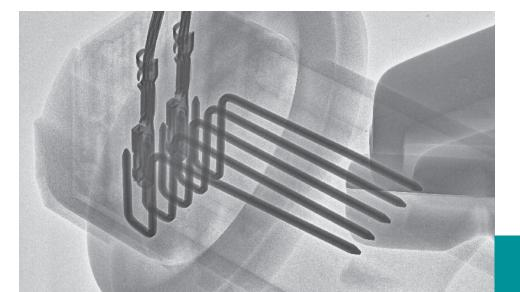
Pioneering software not only detects defects in a machine part, but will also register non-regular changes in the manufacturing processes
